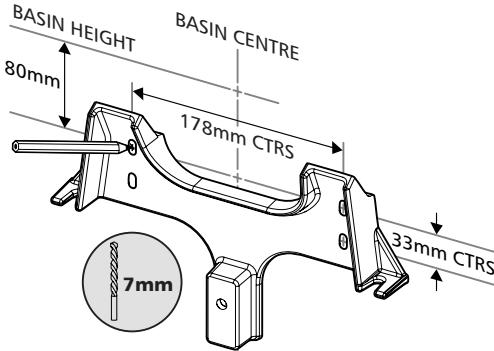
Mark & drill the Ø7mm mounting holes. The top most holes should be marked 80mm below the desired basin height.
