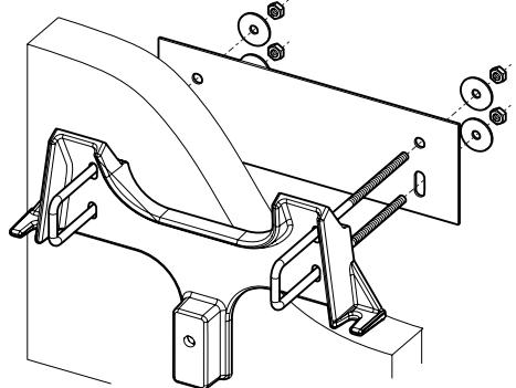
Secure the bracket to the wall using the M6 C-bolts, backplate and M6 penny washers and nuts.
