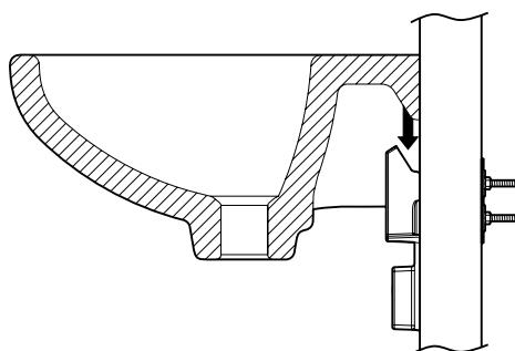
Carefully place the basin onto the bracket ensuring it is fully seated and positioned centrally on the bracket.
