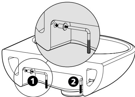
Insert the bushes and then the side anchors into the left and right side holes in the underside of the basin.
