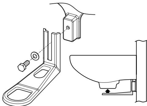
Fit the waste support bracket directly underneath the basin outlet and secure using the brass washer and M10 bolt.
