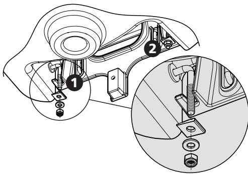
Position the side anchors into the fixing slots and secure using the wedge washer, M8 washer and nyloc nuts.
